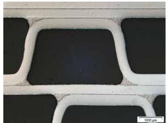
A micrograph of the cross section of a stainless steel EGR cooler brazed with VITROBRAZE VZ2170
